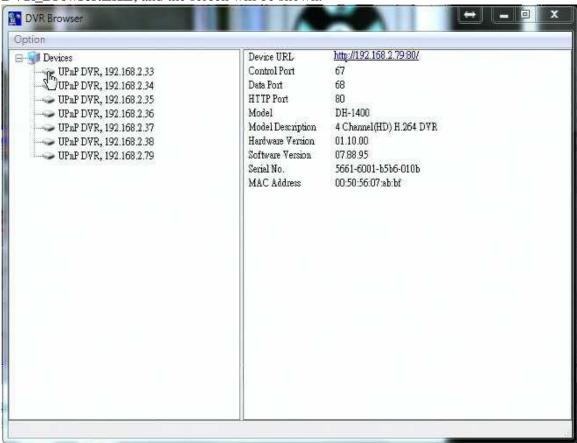
The utility will scan all the DVRs which support UPnP in the LAN. Please select the desired DVR device, and its detailed information will be shown on the right as above. Users can (1) click on the URL to call up IE and logon to the device, (2) select Option->Rescan network, or (3) select Option->Export Device List. The exported device list can be imported to IE software or CMS software in the future.
