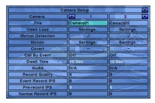
The Camera Setup allows the administrator to define the attributes for each camera. There are up to 8/4 cameras which can be connected to the system.
