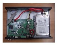
3. Hold the SATA HDD, and use a screwdriver to fix it as shown.
