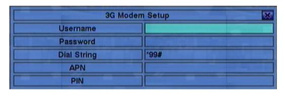
The 3G Modem Setup allows the administrator to set 3G modem related parameters if USB dongle 3G modem is plugged in the USB port.
