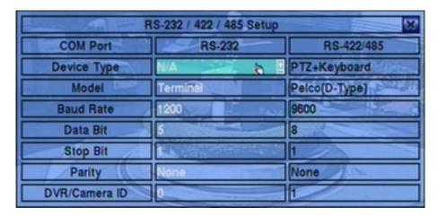
The RS-232/422/485 Setup allows the administrator to setup RS-485 control port. Please refer to the manuals for the connected devices - PTZ cameras or keyboard controllers – to set these items in RS-232/422/485 Setup.
