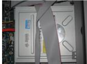
Fig 2-3 Connect the DVD Writer Fig 2-4 Screw the Writer
